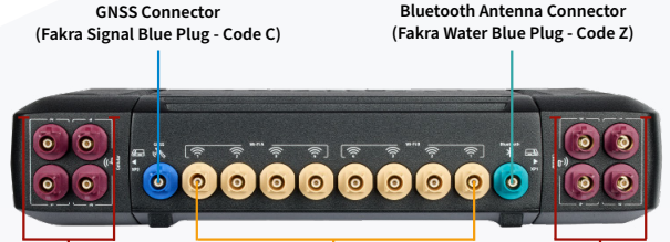
Cellular Antenna (Fakra Bordeaux Violet Plugs - Code D)
