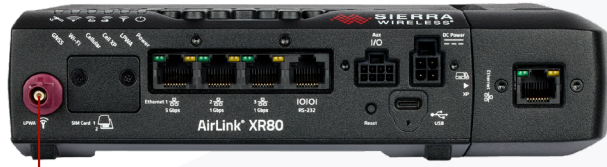
LPWA Antenna (Fakra Bordeaux Violet Plug - Code D)
