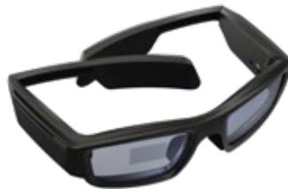
Vibrant full color waveguide display (right eye only)
